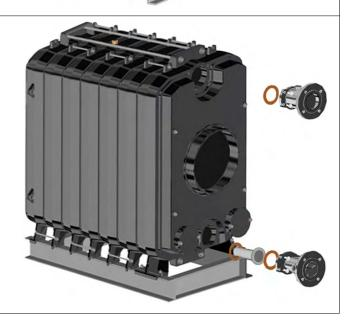
After installation of boiler input and output adaptors, boiler must be tested for leakage by filling water inside without connecting the front burner door ,for 10 minutes under 9 bars pressure .
