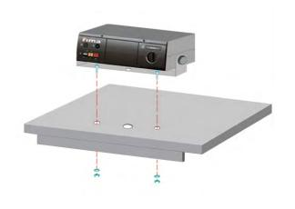
There are three holes on the front cabin sheet. Thermocouples (sensors) of the control panel (thermostat, safety thermostat, thermometer) must be passed through the middle hole. Control panel must be stabilized to the holes on right and left.
