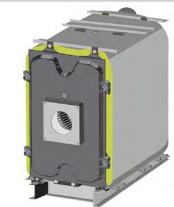
First the holes on the side cabin sheets must be connected to the pins on the assembly legs and than must be connected to cabin sheet assembly ears with M8  $\times$  20 bolts as seen in the picture.
