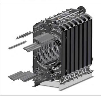
After the installation of the turbulators to the passes boiler burner door must be connected to front section.
